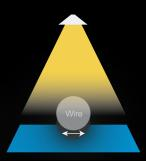
Reduced width and internal reflection decreases shading by a total of 75 %.
