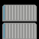
Two half-cells with 12 busbars have the same or even greater output as a full cell with 24 busbars
