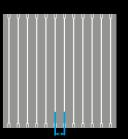
Shorter distance means less resistance and better capture of excited electrons.
