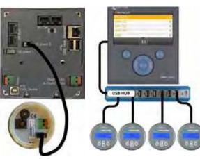
A maximum of four BMVs can be connected directly to the Color Control. Even more BMVs can be connected to a USB Hub for central monitoring.
