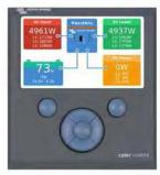
Color Control panel, showing a PV application
